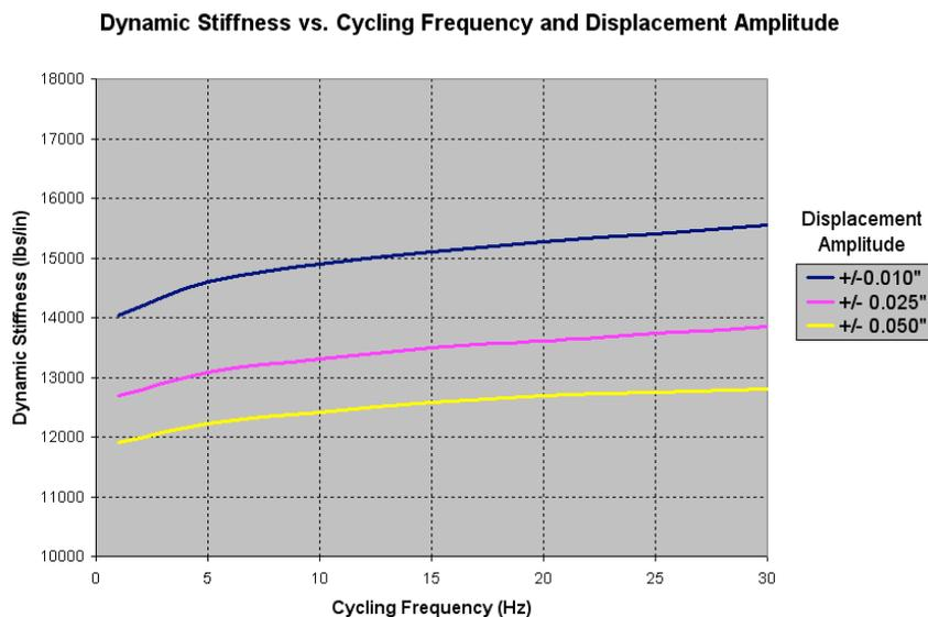
Figure 1 – Effect of strain (amplitude) & strain rate (frequency) on dynamic stiffness
