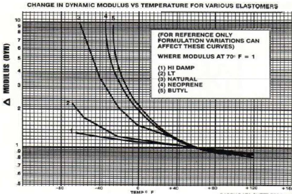
For this comparison, the moduli at room temperature are the same for each of the elastomers. You can see that the stiffening of moduli at low temperature is dramatic. While there is softening at the higher temperatures, it is less dramatic.
