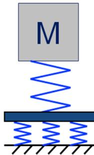
... is that the isolation improves above resonance at 12dB/octave. Thus at high enough frequencies, the isolation could be as much as twice as good as with the single stage system. See Figure 1 on page 2.
