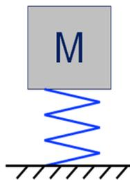
... isolation improves above resonance with increasing frequency. For every 2x increase in frequency, the isolation improves by 6 dB. This is known as a 6dB/octave roll off. The real benefit of a 2-stage mounting system:
